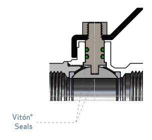
The joint between the main body and lateral adds an o-ring ensuring a mechanical leaktightness..
